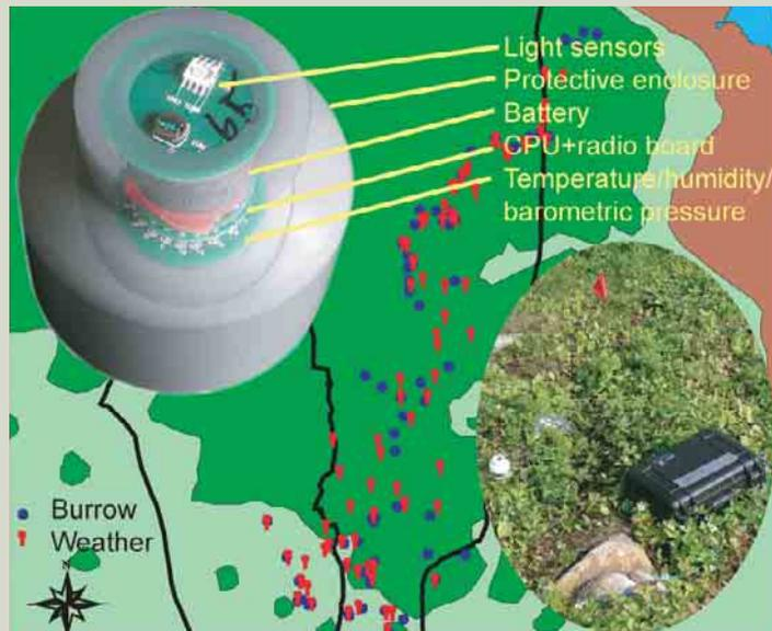
**Great Duck Island deployment; a surface mote (detail) is associated with several underground sensors (red flags) and an infrared camera (black box).**
