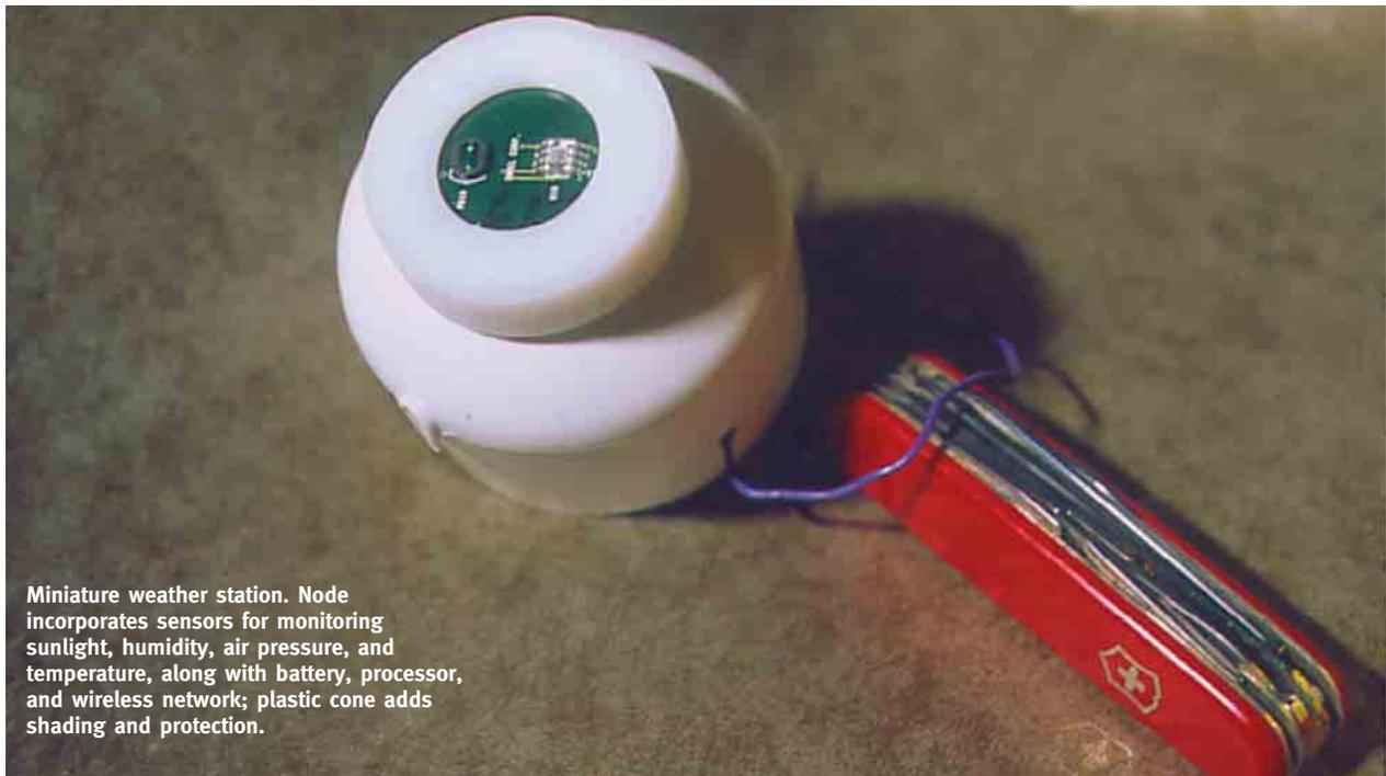
Miniature weather station. Node incorporates sensors for monitoring sunlight, humidity, air pressure, and temperature, along with battery, processor, and wireless network; plastic cone adds shading and protection.
